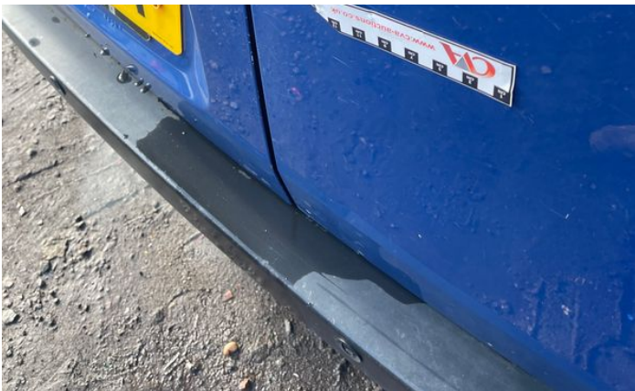
5: Door osf Dented With Paint Damage
